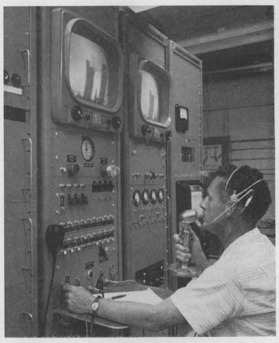
FIRING PANEL and control console for the rocket sled track is operated here by L. R. Myers (1613-4). On the TV monitor screen is a close-up of the Nike Booster rocket on a test stand near the track which was fired shortly after this photo was taken.
